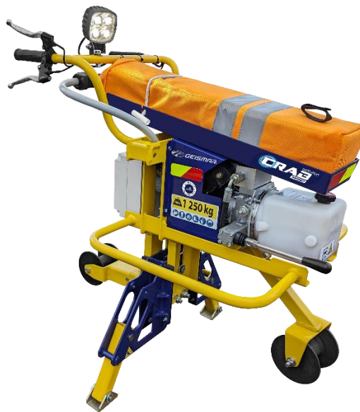
The CRAB mono battery-powered rail lifter is both compact and efficient
